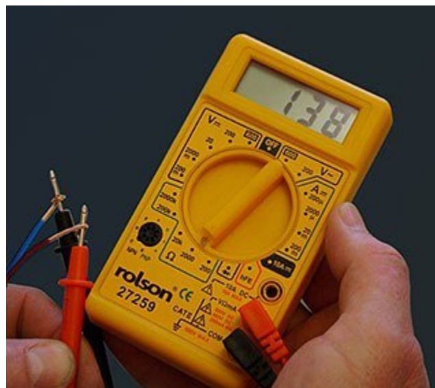
Measuring resistance of a heater (via the leads)
