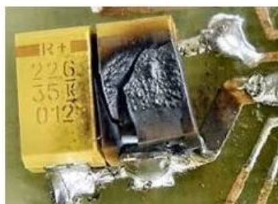
tantalum capacitors can "go up in smoke"
